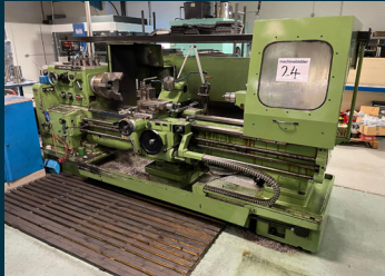
DEAN SMITH AND GRACE Type 2112 x 80 Gap Bed Centre Lathe with SONY Digital Readout. Rebuilt 2000
